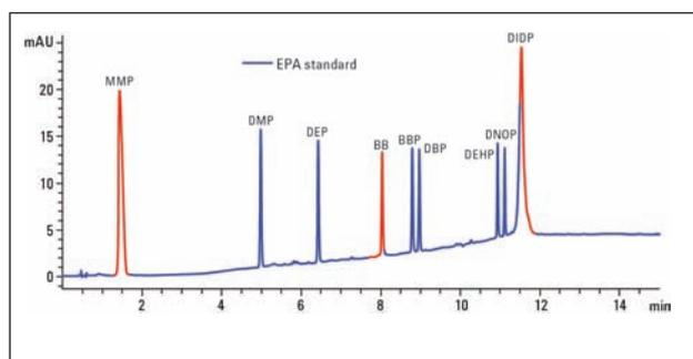
Figure 1. Analysis of phthalates using the phenyl-hexyl column and acetonitrile and methanol in combination.
