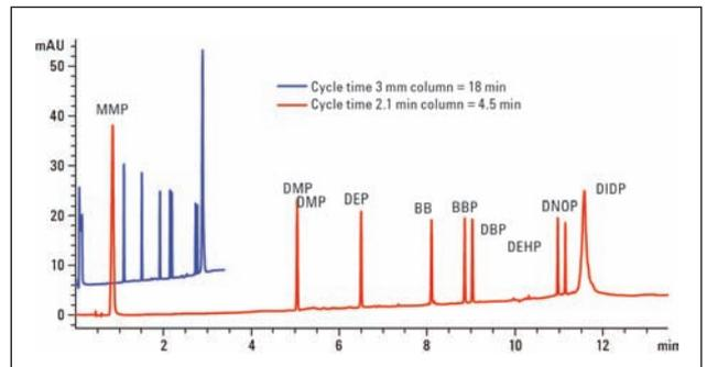
Figure 7. Overlay of chromatograms received from a high resolution and a fast UHPLC run.
