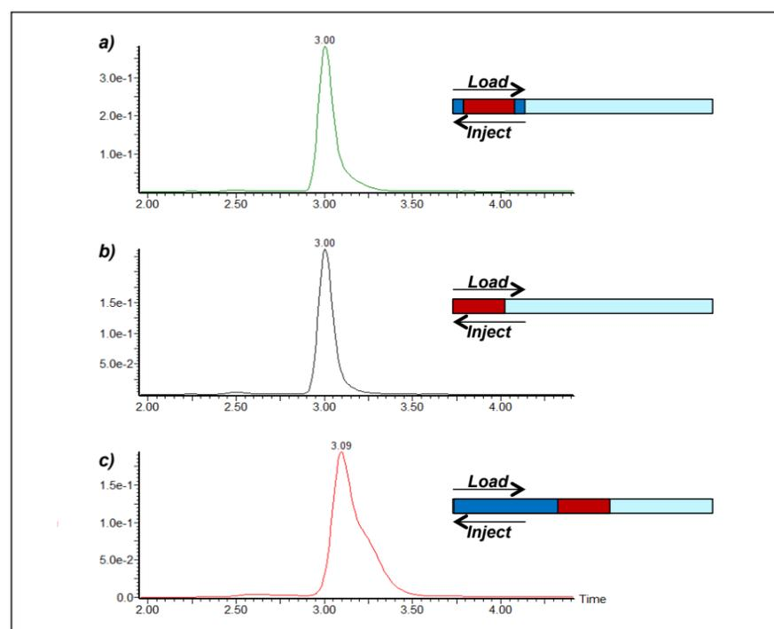
Figure 5. UV chromatograms for coumarin-314 using different injection techniques on the Waters Prep 100 SFC MS system. On the right is the schematic view of the loop for each injection technique. The sample volume is marked in red, pure methanol in dark blue and the modifier in light blue.
