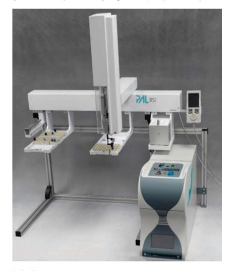
GC-FID analysis. As Omex Environmental is analysing VFAs between C2 and C6, it was proposed that a headspace analysis method could achieve similar results to the liquid:liquid extraction, but with the desired increase in productivity and also the elimination of the use of a solvent, hence the generation of hazardous solvent waste.
