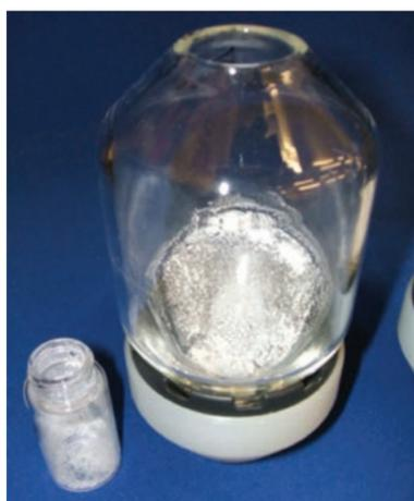
Figure 3. Flask showing sample dried to the sides
