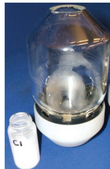
Figure 4. Flask showing minimal sample sticking with added 1,4-dioxane
