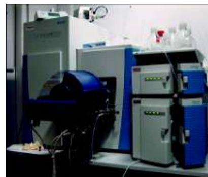
Figure 3. Thermo Fisher Exactive MS and Accela LC with Advion Triversa Nanomate interface.
