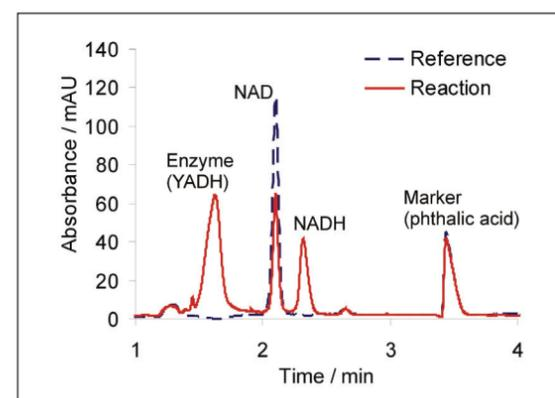
Figure 2b. On-capillary electrophoretic enzyme assay: oxidation of ethanol catalyzed by yeast alcohol dehydrogenase (YADH) involving the cofactor NAD which is reduced to NADH. One capillary used as reactor and the other for reference.
