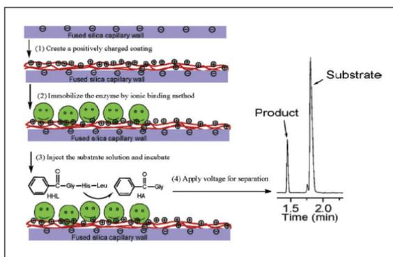
Figure 5. High throughput screening of inhibitors. Schematic representation of on-column immobilized enzyme microreactor prepared by an ionic binding method. Reprinted with permission from Z. Tang and J. Kang, *Anal. Chem.* 2006, 78, 2514. Copyright (2006) American Chemical Society.
