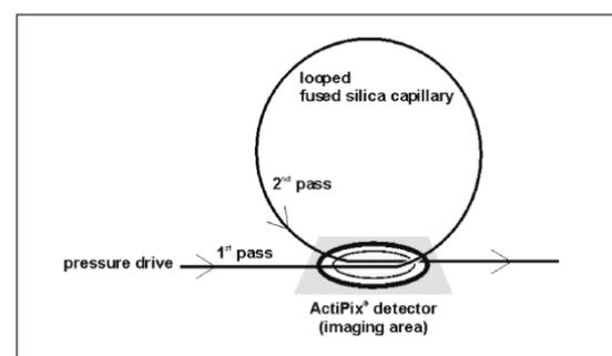
Figure 8a. Capillary loop arrangement for simultaneous UV quantification and sizing.
