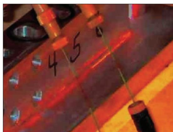
Figure 7. Microfluidic proteomic reactor for on-line protein concentration, reduction, alkylation and digestion. (M. Ethier et al, *J. Proteome Res.* 2006, 5, 2754; picture from: *J. Proteome Res.* 2006, 5, 2750) Courtesy of Daniel Figey.
