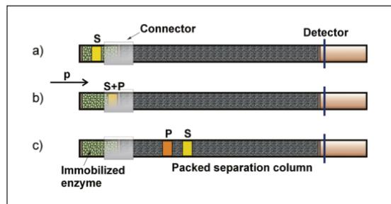
Figure 6. Pressure-driven reaction and separation. Sequence of flow through a packed reactor followed by a packed-bed separation stage: (a) substrate plug injected into the immobilized enzyme zone, (b) pressure-driven flow – substrate/product zone moving towards the separation column, (c) LC separation of substrate and product. PTFE tubing used as zero dead volume connector.
