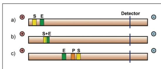
Figure 1. Electrophoretically mediated microanalysis (EMMA): homogeneous reaction/separation sequence using mobility differences. (a) Sandwich injection of reactants, (b) zone overlap, (c) separation of reactant and product.
