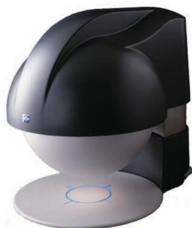
Figure 1: VideometerLab 3: 19 LEDs at separate wavelengths are strobed successively to illuminate the sample with monochrome light. A CCD camera captures an image during each LED strobe period.
