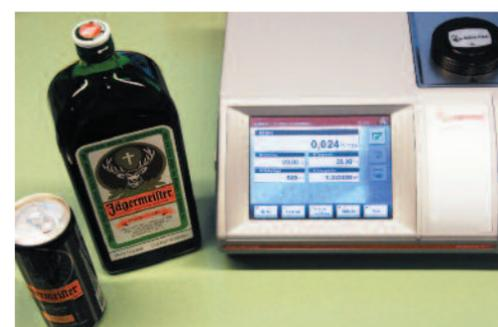
Abbemat 550 refractometer for concentration measurement of liquid sugar and quality control of raw materials and RTDs
