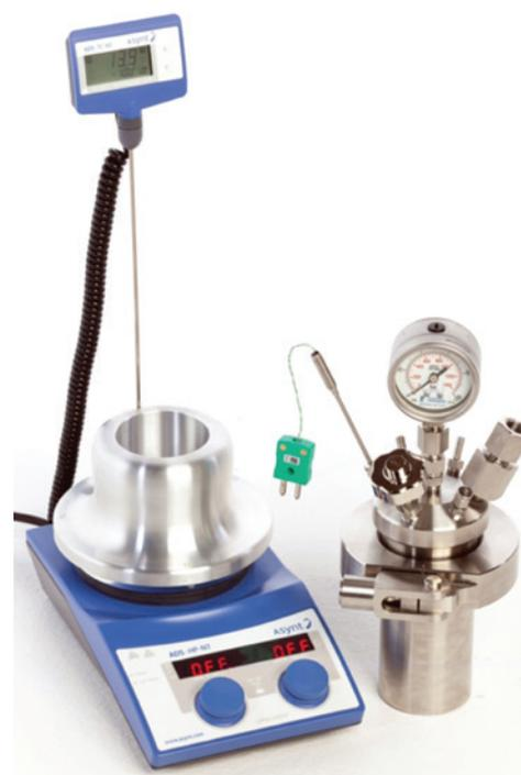
*Figure 3. PressureSyn Reactor on stirrer hotplate*
