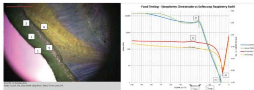
Figure 1: (A) Example of Lyostat analysis of fruit juice. The dried layer is formed at different temperatures (1, 2, 3). The collapse of the product starts at 5. (B) Example of Lyotherm graph of ice cream. Softening events are observed at Z1, whereas at Z2 and D2 there is complete melting
