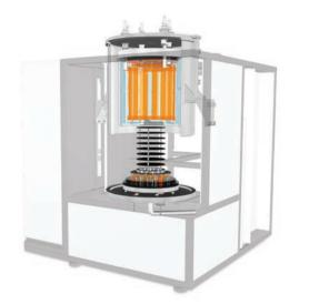
Schematical drawing of the HBO 60 MO/13-1G. The usable volume has a diameter of 400 mm and a heated height of 500 mm. The maximum temperature is 1300°C. Argon can be used to flood the furnace in partial pressure mode.
