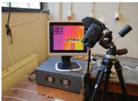
Monitoring a battery cell for hot spots.
