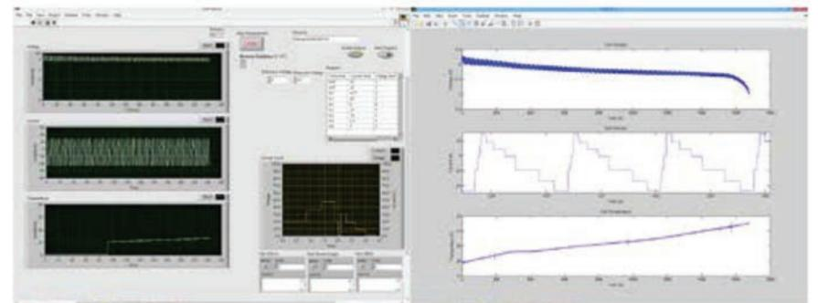
Graphical report of a test cycle of a battery cell test, where temperature values are set out against current and voltage values.
