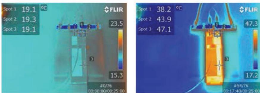
The FLIR T640 is used to detect hot spots of battery cells with different load cases.
