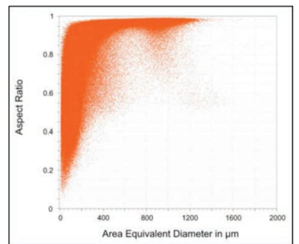
Figure 4: 2D Cloud of the Aspect Ratio over the Area Equivalent Diameter.
