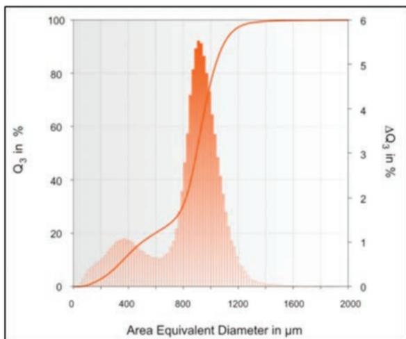
Figure 2: Particle size distribution of a polymer granulate. The size parameter selected is the area-equivalent diameter, i.e. the diameter of a circle with an area equal to the particle cross-section.
