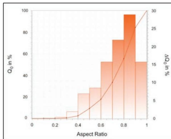
Figure 3: Distribution of the aspect ratio plotted as a cumulative curve (solid line) and as a density distribution (bars). Note the index '0', which indicates a number distribution.
