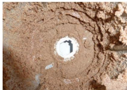
Figure 6. Hazelnuts after 30 seconds grinding in the grinding vessel made of stainless steel.
