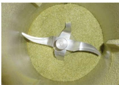
Figure 2. Hops milled at 4,000 rpm, grinding time 15 seconds.
