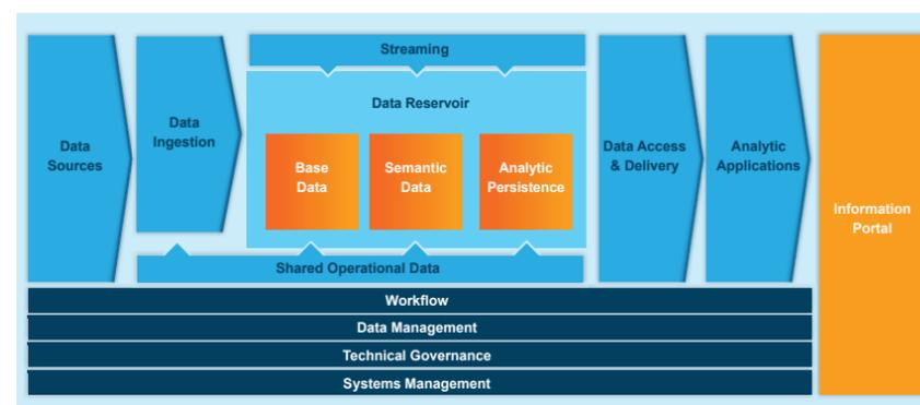
Figure 1: A modern big data and analytics reference architecture defines the boundaries and components for implementing a robust framework required for a data lake.
