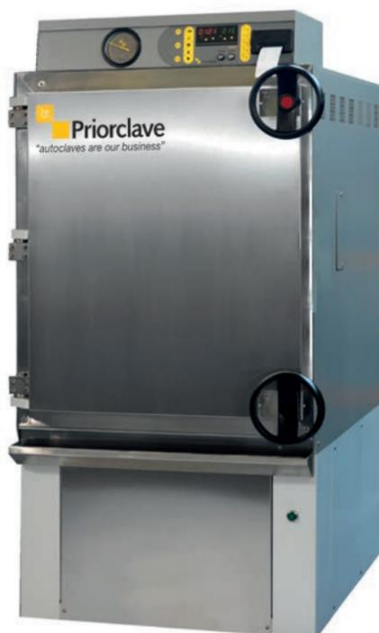
The Priorclave RSC range of front loading autoclaves with their taller, large rectangular steam sterilising chambers has become a popular choice for laboratories undertaking high-volume throughput or frequently tasked with handling taller and bulkier items. Despite the extra-large chamber these autoclaves require only a relatively small floor area.
