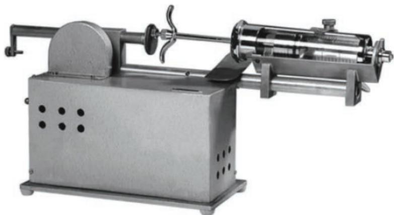
Figure 1. A simple infusion device designed by Dr Hess possessing primitive gearing
