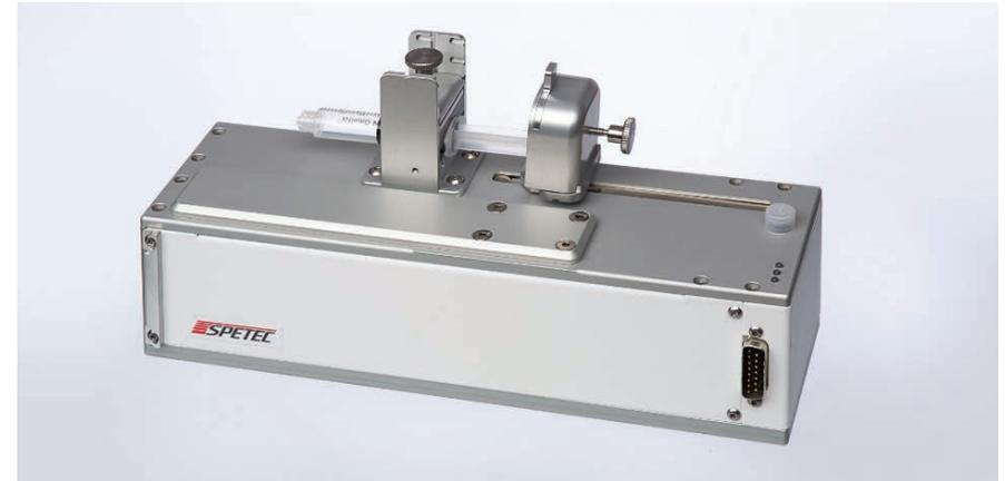
Figure 3. The SYMAX syringe pump
