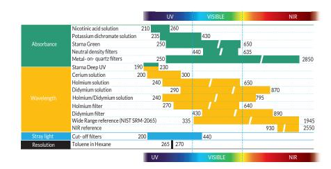
Figure 1. Wavelength ranges of Certified Reference Materials
