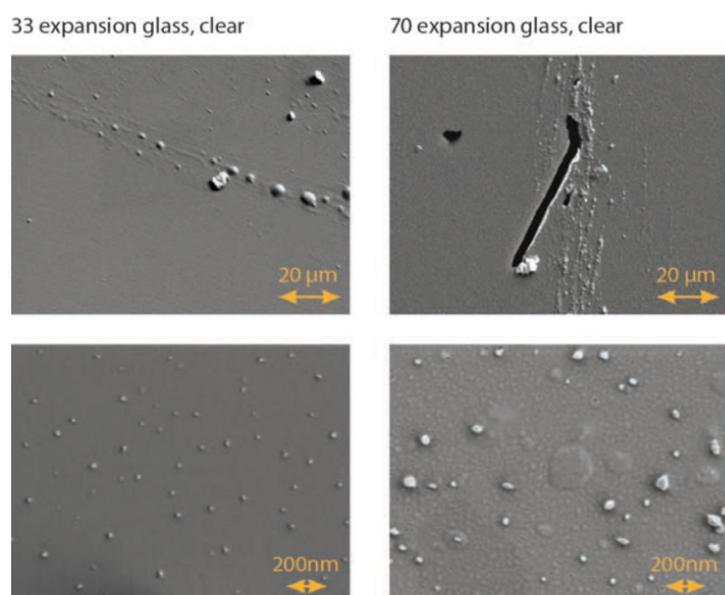
Figure 1. Glass quality comparison showing 1st hydrolytic glass, types 33 vs 70.
