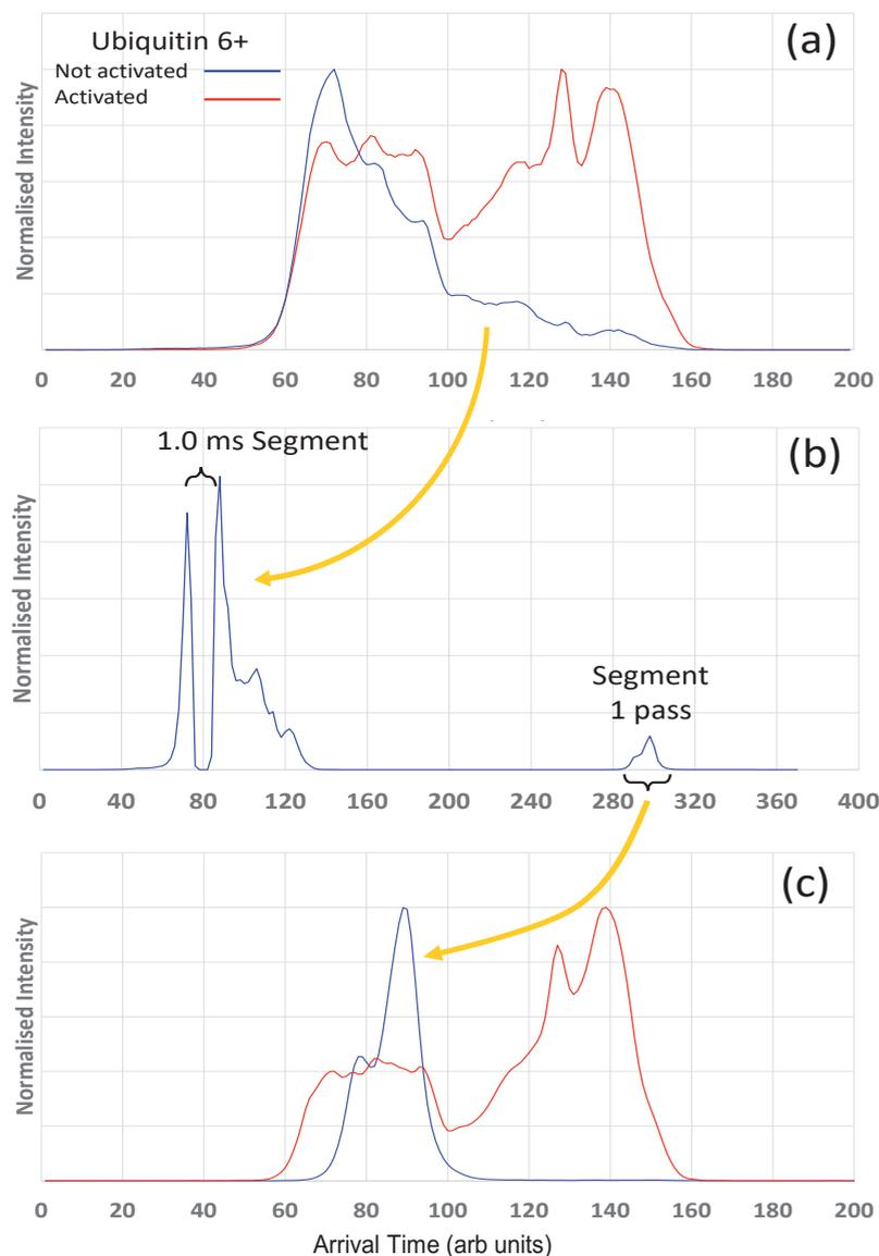
Figure 3. Arrival Time plots for Ubiquitin ( $(M+6H)^{6+}$ ) (a) single pass separation (b) 1 ms segment selected from single pass ions then a single pass on the selected ions ( $IMS^2$ ) (c) expanded view of selected segment plot.
