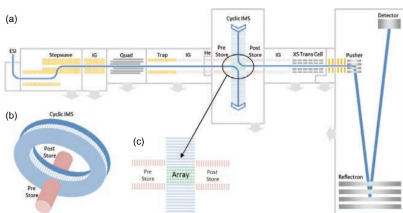
Figure 1. (a) Instrument schematic showing the Q-IM-ToF geometry. (b) Graphic showing the orthogonal arrangement of the Cyclic IMS and neighbouring ion optics. (c) Multi-function region (Reproduced with permission from ref [1]. Copyright 2019, Ujma et al.)
