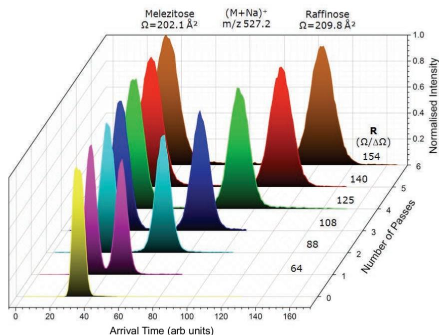
Figure 2. Cyclic IMS separation of two isomeric trisaccharides, Melezitose and Raffinose as a function of the number of passes (where R is the measured resolving power). The two species are separable because of their differing CCS (Ω) values.
