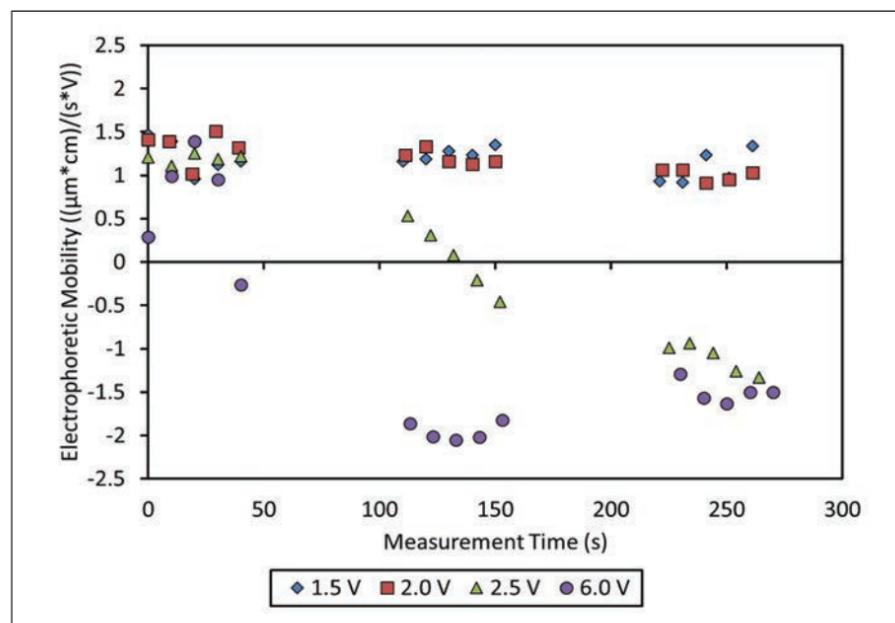
Figure 4. Automated mobility measurements reveal that aluminium adjuvant mobility turns negative at higher voltage, indicating that reduction has occurred.
