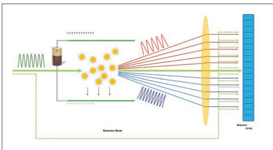
Figure 2. Modern MP-PALS systems allow users to measure the electrophoretic mobility of delicate nanoparticle and protein formulations quickly and non-destructively.
