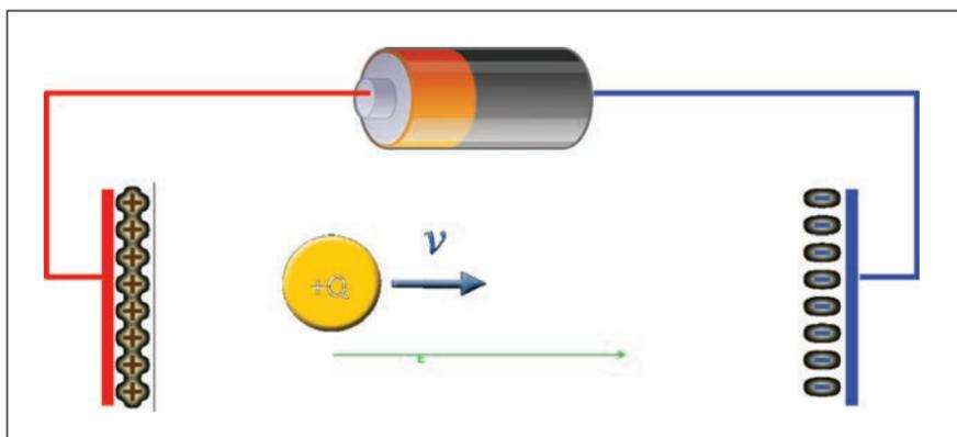
*Figure 1. Applying an electric field to protein particles in formulation enables the measurement of electrophoretic mobility, a key stability predicting parameter.*
