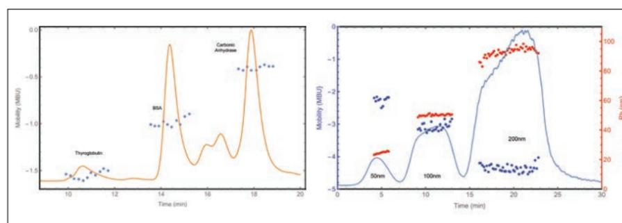
Figure 5. Combining concentration and mobility data for each point allows users to generate a high-resolution size-mobility distribution plot. Left: proteins separated by SEC; right: latex spheres separated by FFF.
