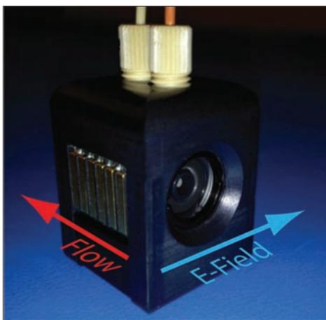
Figure 3. The sample flow through the cell is perpendicular to the electric field allowing for online coupling of MP-PALS to separation techniques.
