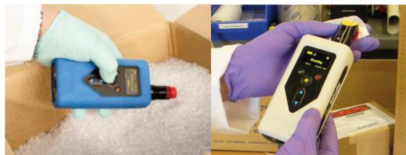
Figure 4: RAPID-ID (left) and PHARMA-ID (right) handheld Raman spectrometers from DeltaNu
