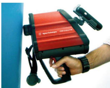
Figure 2: ExoScan 4100 handheld FTIR
