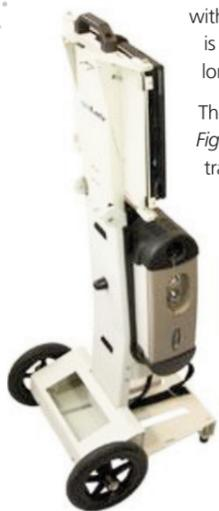
from ASD Inc is shown (figure 3), this research grade instrument can be operated with a selection of fibre optic probes, both reflectance and transmission, and is ideal for field measurements since operation is truly independent using long life battery packs.
