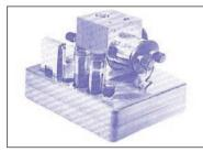
Figure 1: An early photometer from Evans Electroselenium Ltd
