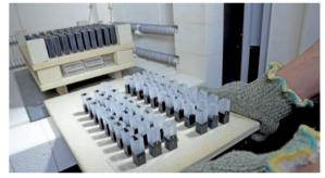
5 Figure 3: Cuvettes being stacked in an oven for the fusion process
