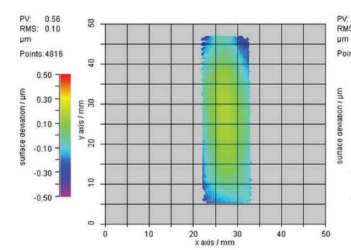
Figure 4 (a) surface scan of a quality cuvette
