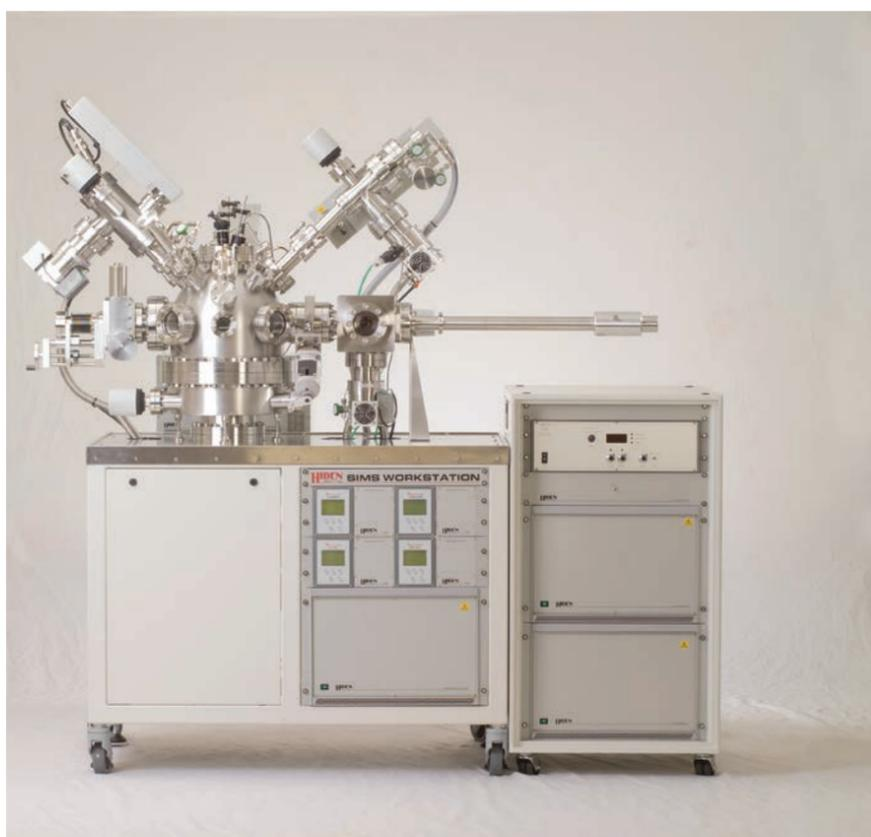
SIMS Workstation for thin film depth profiling
