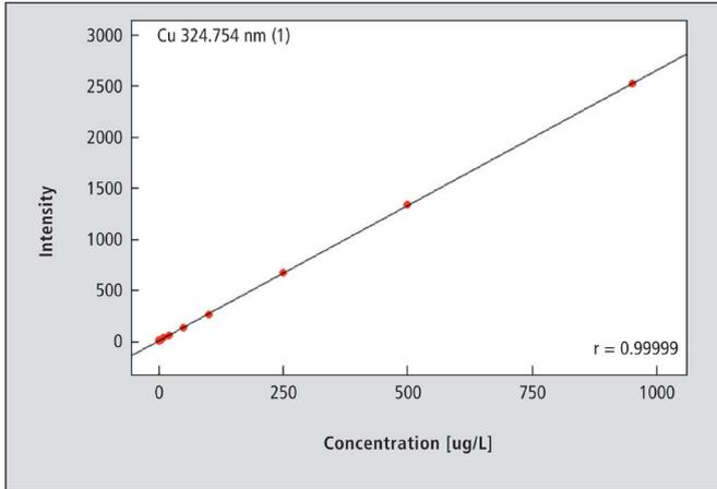
Figure 2. Copper Calibration
