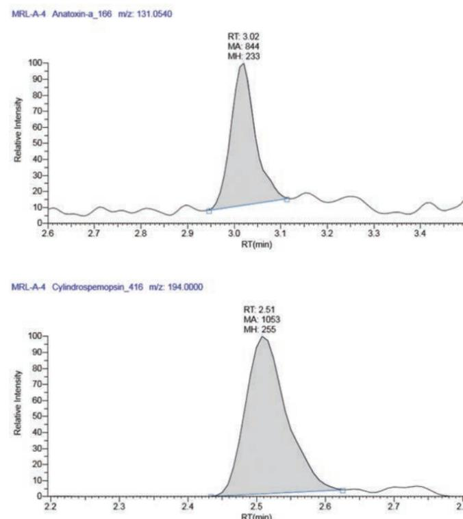
Figure 3. 5 µL injection volume chromatograms, (A) anatoxin-a, (B) cylindrospermopsin.
