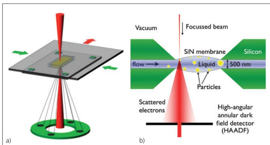
Figure 4. Schematic of the fluid-cell scanning transmission electron microscopy geometry. (a) The scanned electron beam passes through two SiN membranes which separated the fluid from the microscope vacuum. Two inlet ports and one outlet port allow for the independent introduction of fluids and the time resolved observation of dynamic processes. (b) A cross-sectional schematic of the arrangement of the SiN membranes.
