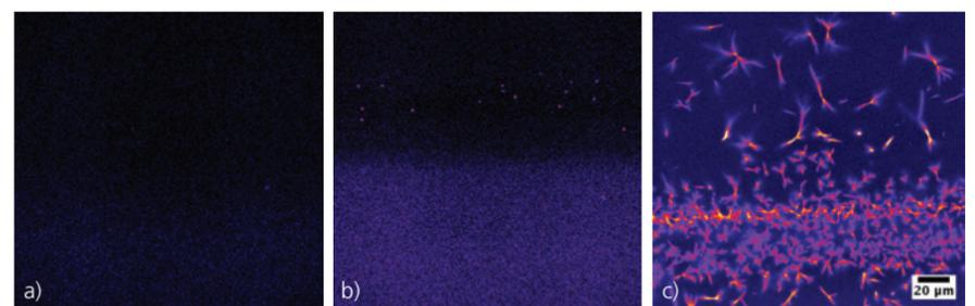
Figure 2. Fluid cell/ASEM studies of back-scattered electron intensity dependent on concentration. (a) top: water, bottom: 25 mM  $\text{Ba}^{2+}$  solution, (b) top: water, bottom: 100 mM  $\text{Ba}^{2+}$  solution, (c) top: 10 mM  $\text{CO}_3^{2-}$  solution, bottom: 100 mM  $\text{Ba}^{2+}$  solution leading to precipitation of  $\text{BaCO}_3$ .
