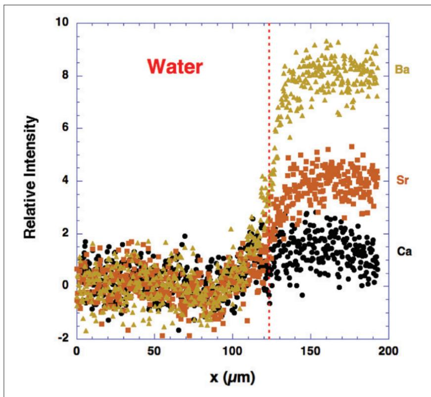
Figure 3. BSE contrast measured using line scans across the water/salt solution boundary for different earth alkaline metal ion solutions ( $\text{Ba}^{2+}$ ,  $\text{Sr}^{2+}$  and  $\text{Ca}^{2+}$ ) showing the impact of the atomic number  $Z$  on the contrast between water and solution.
