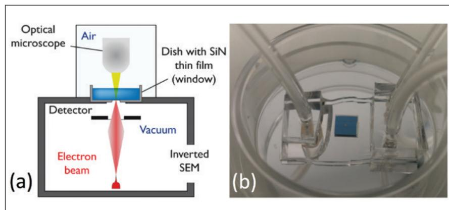
Figure 1. (a) Schematic of the atmospheric SEM, (b) integrated microfluidic channel in Petri dish used for fluid analyses in ASEM.
