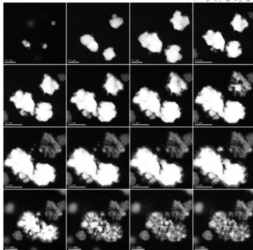
Figure 5: Investigation of  $\text{CaCO}_3$  precipitation in the presence of the nacre protein AP7 by fluid cell STEM showing the time dependence of protein agglomeration, precipitation of calcite and subsequent dissolution under reduced electron beam irradiation. The time frame from the first to the last image of the sequence is 1200 s.
