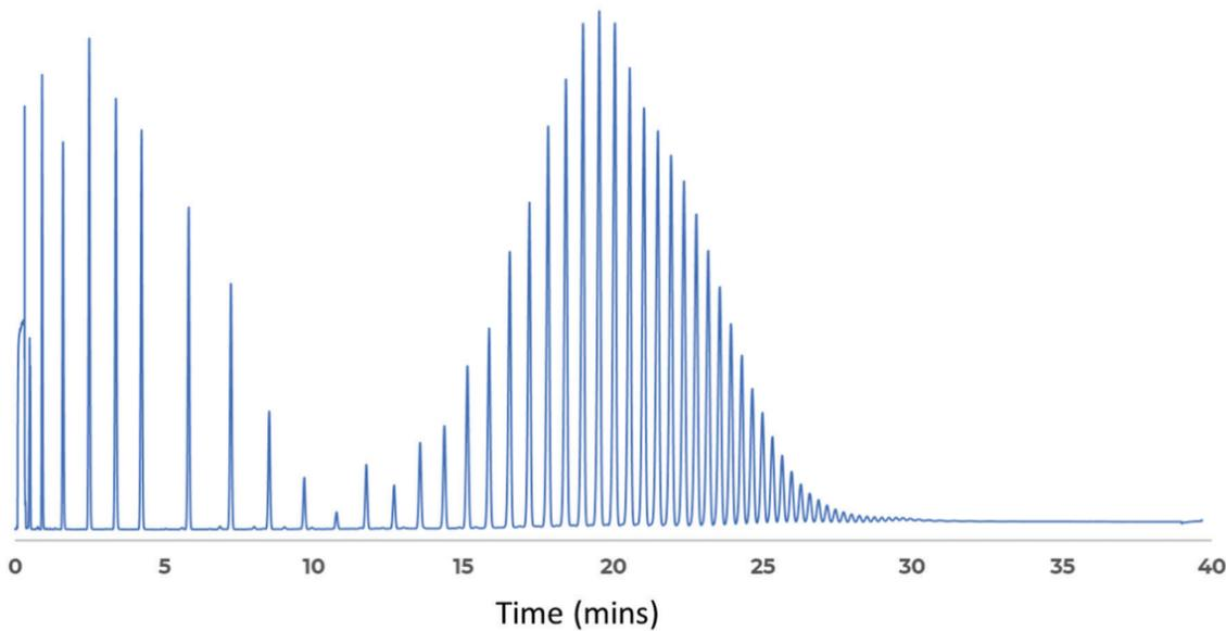
Figure 1. Chromatogram of D7169 calibration standard (C<sub>5</sub>-C<sub>100</sub>)
