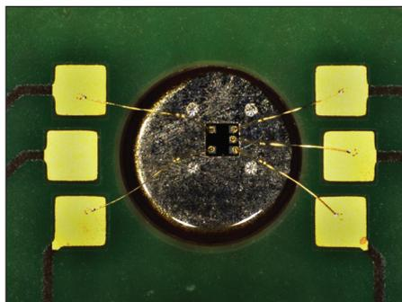
Figure 5. Magnification of a strain gauge sensor. The strain gauge is attached to the surface of the MMF structure and the board of the hybrid structure.
