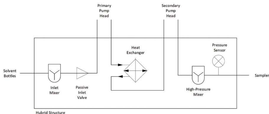
Figure 6. Diagram of pump head manifold. This hybrid structure is used before, between, and after the primary and secondary pump head of an HPLC quaternary pump and serves as a connecting manifold. In this setup, the device connects a gradient valve to the primary via a low pressure mixer and a passive inlet valve; the primary to the secondary via a heat exchanger and the secondary to the system via a mixer and a pressure sensor.
