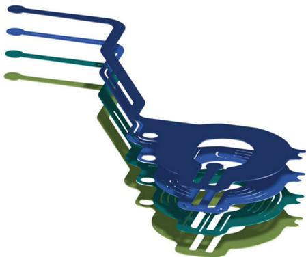
Figure 2. Individual layers of the high pressure heat exchanger prior to bonding the individual layers. Each layer has a sub-set of channels which, when combined, result in the complete flow channel for the device.
