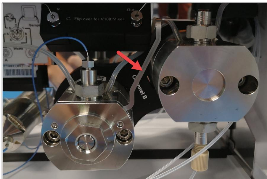
Figure 1. Example of a current application for MMF devices. Conventional pump head that is equipped with an MMF heat exchanger.
