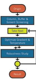
Picking parameter ranges for screening is only the start of the experimental work. A rational approach to method development explores the selected parameter space to find optimal and robust areas.
