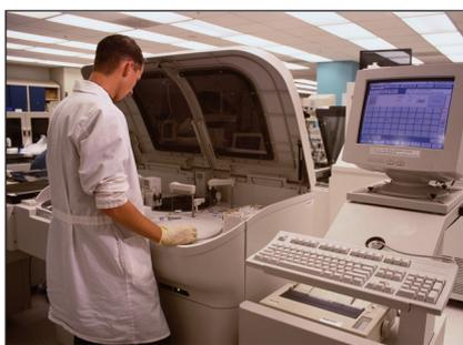
But there are even further obstacles. Often laboratory benches are positioned against walls, and back to back with each other. This not only makes access very difficult for service engineers performing instrument maintenance, but is not ideal from the instrument function perspective. A lack of space behind instruments which generate or use heat, can minimise the cool down efficiency of the fans placed inside them to precisely control this.
