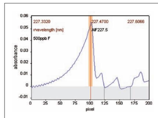
Figure 1. Molecular absorption spectrum of AlF by wavelength resolution in the region of 227.47nm, injection of 10ng F
