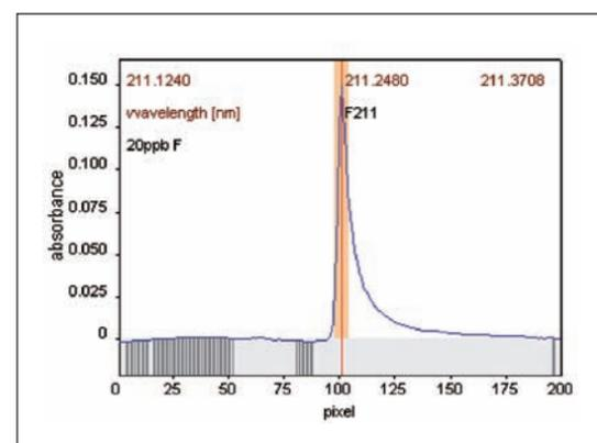
Figure 2. Molecular absorption spectrum of GaF by wavelength resolution in the region of 211.248nm, injection of 10ng F
