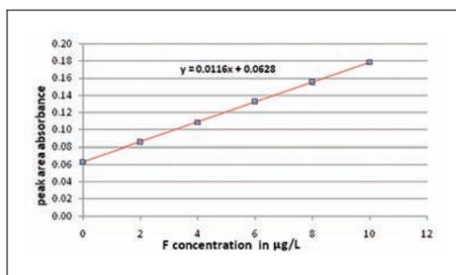
Figure 4. F calibration curve using GaF molecular absorption at a wavelength of 211.248nm: 2 – 10µg/L F, 20µL sample injection
