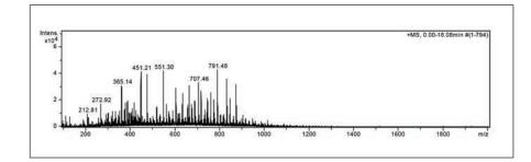
Figure 6. The average mass spectrum of HPLC grade water versus LC-MS grade acetonitrile (Riedel-de Haën 34967) is shown. In conclusion to the measurement above the contamination originates only from the HPLC grade water.
