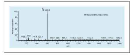
Figure 1. The Reserptne test shows a reserptne spectrum measured in Methanol; no signals should be greater than  $[M+H]_{+} = 609$  (100ppb reserptne; ESI, positive mode).
