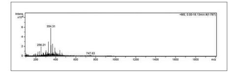
Figure 5. The average mass spectrum of LC-MS grade Water and LC-MS grade Acetonitrile (Riedel-de Haën 39253 versus 34967) is shown. Figure 6 is the direct comparison with an HPLC grade water.
