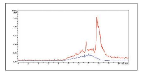
Figure 3. HPLC baseline produced by a gradient from 100% Water (Riedel-de Haën LC-MS CHROMASOLV 39253) to 100% acetonitrile (Riedel-de Haën LC-MS CHROMASOLV 34967) blue chromatogram. The red chromatogram is the same gradient using basic HPLC grade water and acetonitrile. The contamination originates only from the HPLC grade water.
