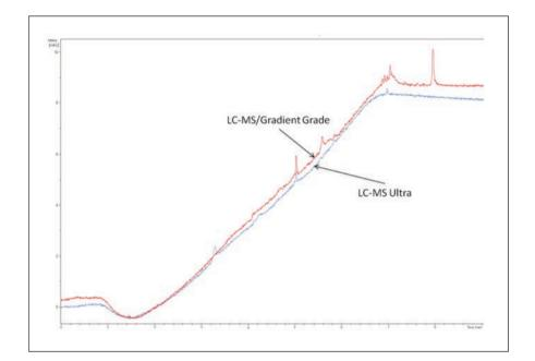
Figure 2. Comparison LC-MS/Gradient Grade under UHPLC Conditions
