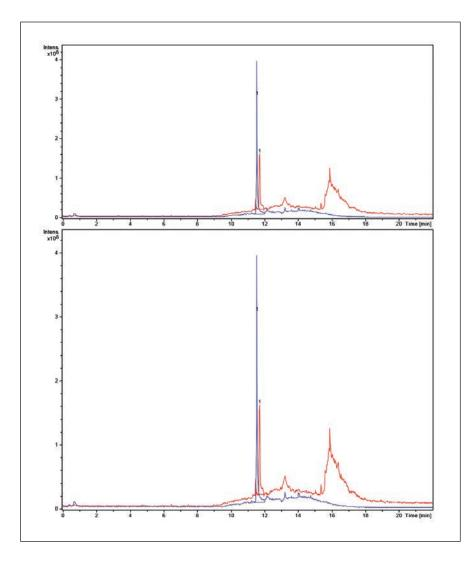
Figure 4. In this example the chromatogram shows a 5 ppm injection of reserpine using the same gradient conditions. The red line shows HPLC grade water / acetonitrile and the blue line shows LC-MS water / acetonitrile (Riedel-de Haën 39253 and Riedel-de Haën 34967).
