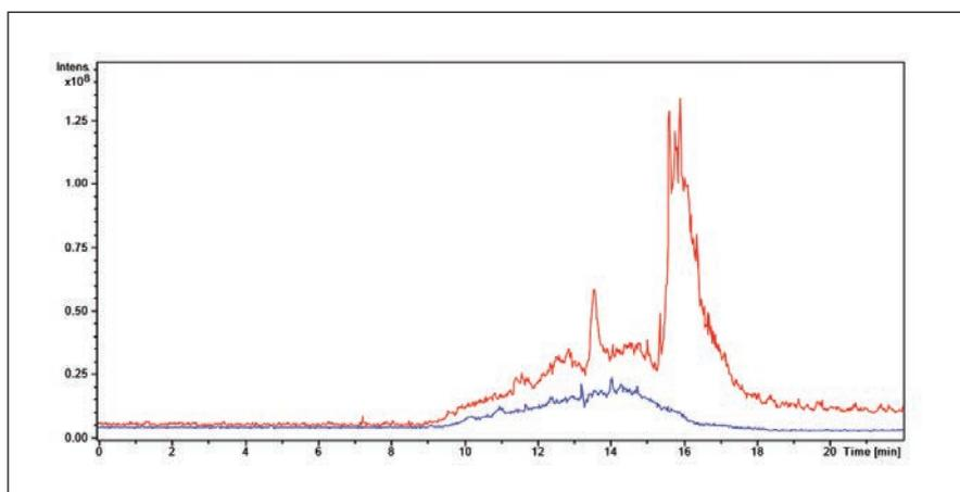
Figure 3. HPLC baseline produced by a gradient from 100% Water (Riedel-de Haën LC-MS CHROMASOLV 39253) to 100% acetonitrile (Riedel-de Haën LC-MS CHROMASOLV 34967) blue chromatogram. The red chromatogram is the same gradient using basic HPLC grade water and acetonitrile. The contamination originates only from the HPLC grade water.
