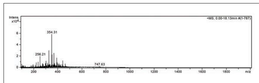
Figure 5. The average mass spectrum of LC-MS grade Water and LC-MS grade Acetonitrile (Riedel-de Haën 39253 versus 34967) is shown. Figure 6 is the direct comparison with an HPLC grade water.
