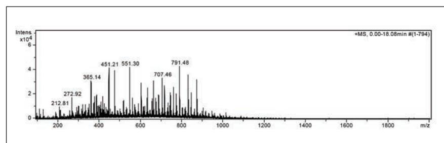
Figure 6. The average mass spectrum of HPLC grade water versus LC-MS grade acetonitrile (Riedel-de Haën 34967) is shown. In conclusion to the measurement above the contamination originates only from the HPLC grade water.
