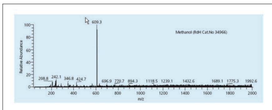
Figure 1. The Reserpine test shows a reserpine spectrum measured in Methanol; no signals should be greater than  $[M+H]^+ = 609$  (100ppb reserpine; ESI, positive mode).
