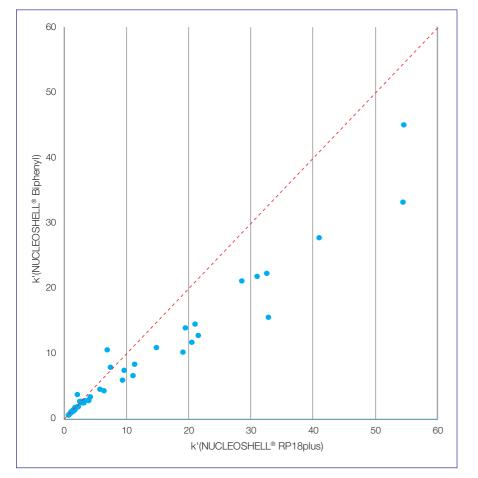
Figure 4. Comparison of NUCLEOSHELL® RP 18plus and NUCLEOSHELL® Biphenyl (acetonitrile/water).
