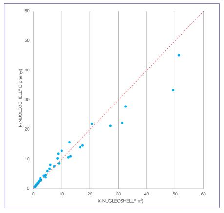
Figure 3. Comparison of NUCLEOSHELL<sup>®</sup>  $\pi^2$  and NUCLEOSHELL<sup>®</sup> Biphenyl (acetonitrile/water).
