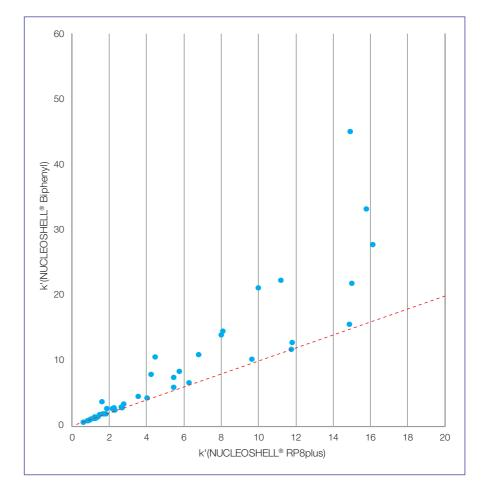
Figure 5. Comparison of NUCLEOSHELL® RP 8plus and NUCLEOSHELL® Biphenyl (acetonitrile/water)
