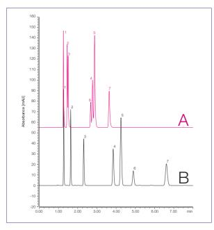
Figure 9: Separation of a test mixture on NUCLEOSHELL® RP 8plus and NUCLEOSHELL® Biphenyl
