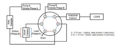
Figure 2: Flow diagram of online SPE-LC-MS/MS system for immunosuppressants.
