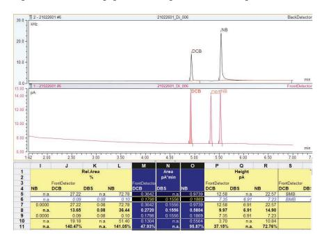
Figure 4. Analysis using Gemini Confirmation mode. A standard mixture containing dichlorobenzene (DCB), dibutylsulfide (DBS), and nitrobenzene (NB) is analysed using GC-ECD (top) and GC-FID (bottom). Data obtained on the two parallel channels are collected within a single data file and the results can be visualised by clicking on the respective chromatogram (here the front channel chromatogram is selected). Processing methods can be applied to both channels or single channels only.
