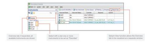
Figure 5. Screenshot of the Overview tab in Chromeleon CDS 7.3. Lines highlighted in green refer to a system running samples on both injectors in High-throughput mode.
