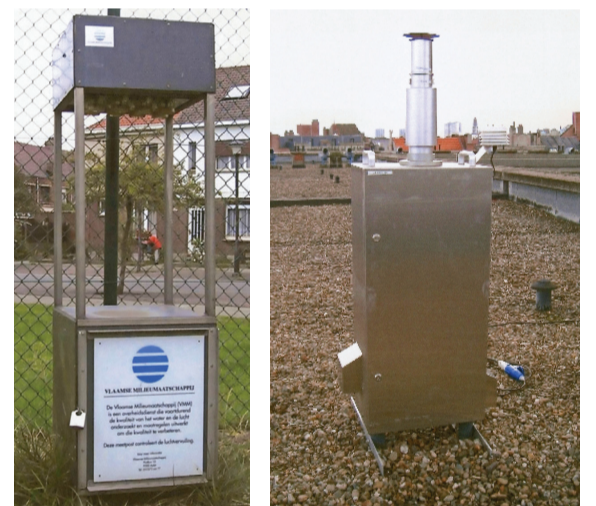
Figure 2: VMM's samplers: Pourbaix low volume (left) and Leckel PM10 (right)
