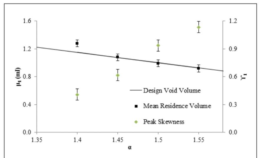
Figure 6. Comparison of theoretical and experimentally determined void volumes and peak skewness of RTD profiles.
