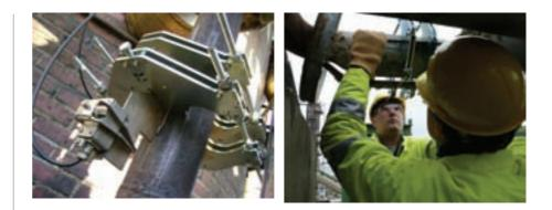
plates radiates enough heat to keep the temperature at the mounting point of the transducers within the permissible range. Simultaneously, the coupling plates ensure the needed acoustical contact between pipe and transducer. The mechanically robust mounting fixture maintains a high contact pressure. Specially designed metal foils ensure optimal contact and long-term stability.
