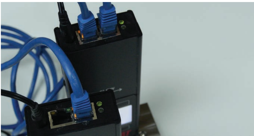
Figure 1: Device level ring connections for Ethernet/IP devices. Image source: Alicat Scientific, Inc.
