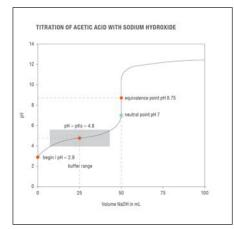
Figure 1. Titration of acetic acid against a strong base (NaOH). In the beginning of the titration the solution is acid. While adding more and more NaOH the pH slightly increases, then makes a steep rise, passes the equivalence point (turning point), and finally increases slightly again when the solution is alkaline (surplus of NaOH).
