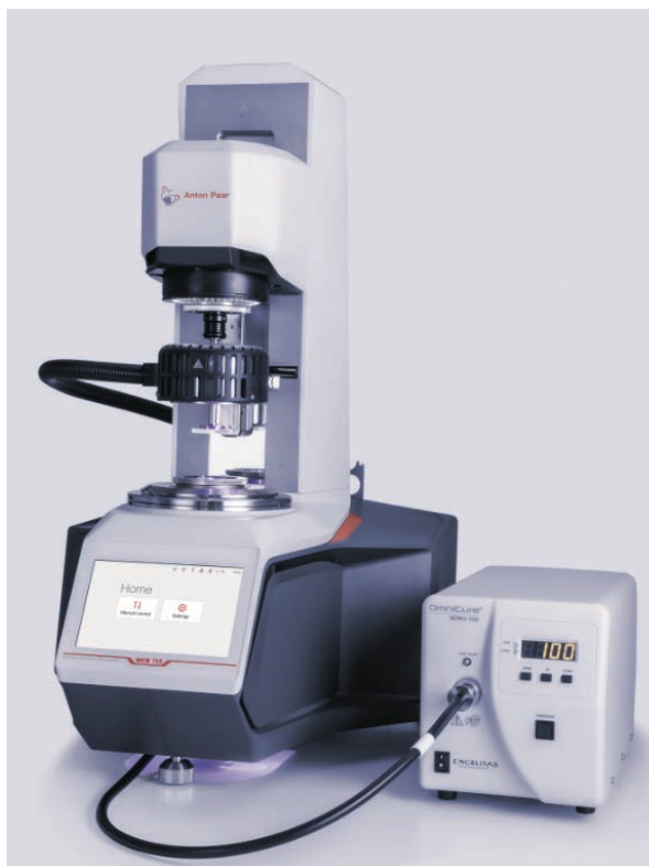
Figure 7: Example of a UV-curing experiment on a nail polish, where the storage and loss moduli are monitored in real time as the material solidifies. In this configuration, UV light is directed onto the sample from below through a transparent glass plate, enabling precise and reproducible curing under controlled rheological conditions.
