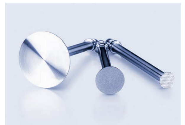
Figure 6: To avoid wall slip, measuring systems with rough surfaces can be used: left: smooth; middle: sandblasted; right: perforated surfaces.
