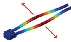
Figure 3b. Working principle of an X-oscillator.
