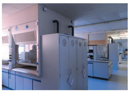
Type 90 safety storage cabinets according to BS EN 14470-1 in a laboratory at Sussex University
