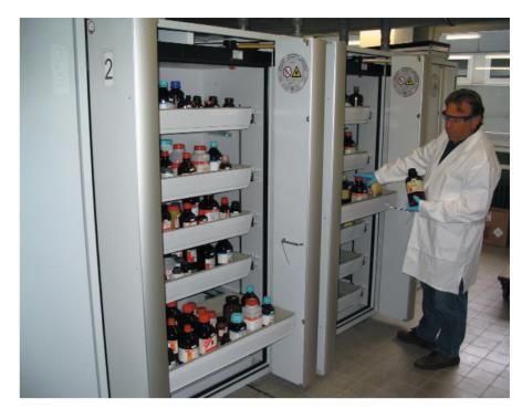
Safety storage cabinets according to BS EN 14470-1 in a laboratory at Gießen University
