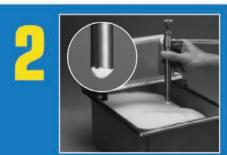
**DIP THE GUN** into the product trough. Powder is instantly picked up into the barrel at a controlled, even density.
