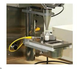
powders. However, their downfall lies in the additional attention required for a steady and even feeding process. Failure to do so could result in unreliable accuracy levels as well as possible product damage due to the compression inside of the cylinder and auger.
