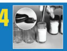
**INSERT THE GUN** into the mouth of the container to be filled. Depress the foot switch. Vacuum changes to gentle pressure, discharging another perfect, dust-free dose.
