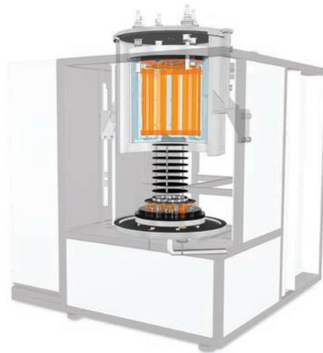
*Schematic drawing of the HBO 60 MO/13-1G. The usable volume has a diameter of 400 mm and a heated height of 500 mm. The maximum temperature is 1300°C. Argon can be used to flood the furnace in partial pressure mode.*
