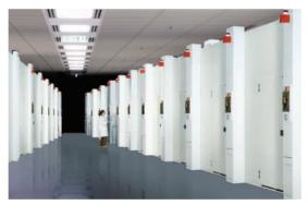
Our Stability Storage suite of rooms and chambers are held at temperatures ranging from  $-86^{\circ}$ C up to  $+60^{\circ}$ C and at humidity levels between 15% and 95% relative humidity – and we routinely provide all ICH conditions.
