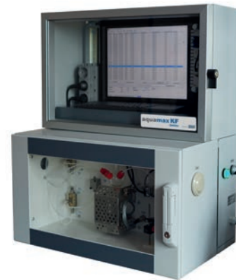
Figure 6: Aquamax KF Online for continuous online monitoring of water content in oil samples.
