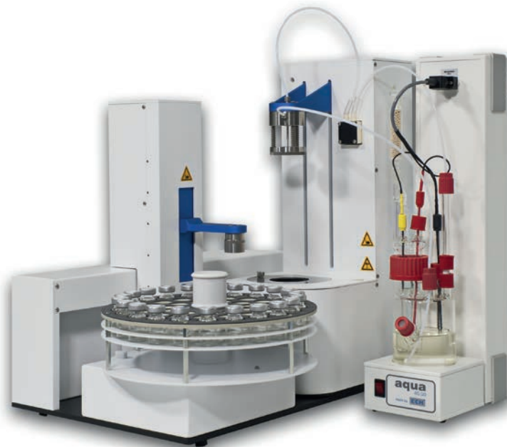
Figure 2: AQUA 40.00 Vario PLUS for water determination in solids and highly viscous samples.
