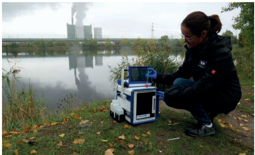
Figure 3: Measurements in the field without stabilizing reagents.
